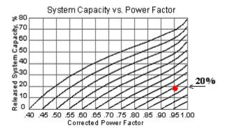
The corrected system is now capable of supporting 960 KW of productive power.
