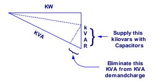
The capacitor performs the function of an energy storage device. By supplying KVAR right at the load, the capacitors relieve the utility of the burden of carrying the extra KVAR. This makes the utility transmission/distribution system more efficient, reducing cost for the utility and their customers.
