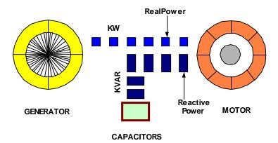
In the illustration above, addition of the capacitor has improved line power factor and subtracted the non-working current from the lines. Rather than transfer energy back and forth between load and generator, the reactive energy to supply the magnetizing current is now stored in a capacitor at the load, thus reducing the distribution requirements for excessive current. This reactive current supplied by the capacitor rather than the utility.
