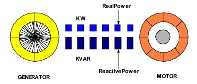
The figure below shows the results of installing a capacitor near the same motor to supply the magnetizing current required to operate it. The total current requirement has been reduced to the value of the useful current only, thus either reducing power cost or permitting the use of more electrical equipment on the same circuit.
