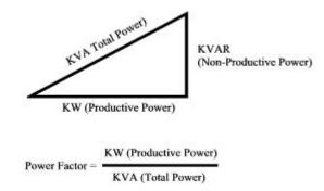
The cosine of the phase angle Ø between the KVA and the KW components represents the power factor of the load. KVAR represents the non-productive reactive power and Ø is lagging phase angle.
