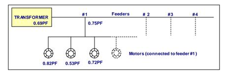
Measuring power factor is a costly procedure when it is required to shut the load down and connect in a metering system to measure the current, voltage and power. So as to avoid the costly shutdown and time-consuming measurement, it is preferable to use a clamp on power factor meter.
